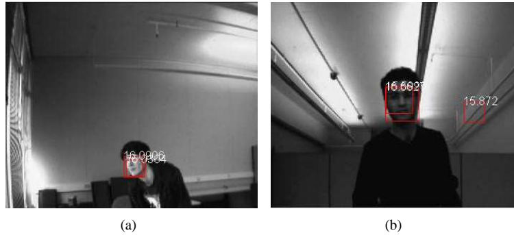
Figure 4: Sample output from a modified Viola-Jones face detector. Faces are denoted with boxes. Image (b) shows how texture in the background can occasionally be detected as a false positive.
