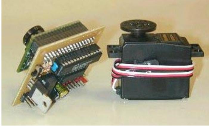
Figure 1: The microcontroller board mated with the CMOS camera module. A standard size hobby servo is shown for scale.
